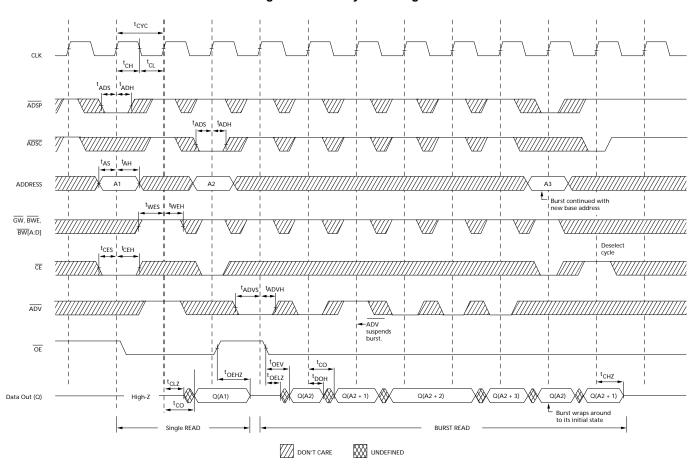
18. On this diagram, when  $\overline{CE}$  is LOW,  $\overline{CE}_1$  is LOW,  $\overline{CE}_2$  is HIGH and  $\overline{CE}_3$  is LOW. When  $\overline{CE}$  is HIGH,  $\overline{CE}_1$  is HIGH or  $\overline{CE}_2$  is LOW or  $\overline{CE}_3$  is HIGH.
